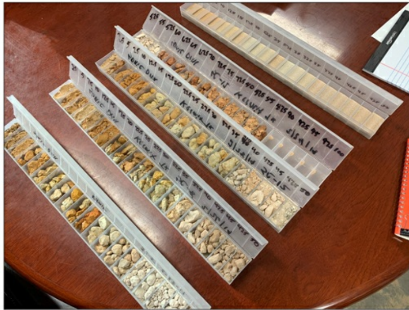
Figure 5.1: 2.5 ft Interval Chip Trays from Various Rotosonic Drill Holes
